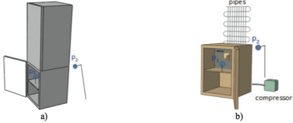
Fig. 1. The schematics of a) the household test refrigerator and b) the designed test rig
