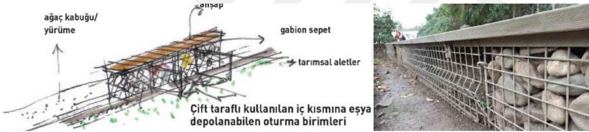
Figure 70. (Left) Drafts for the seating and storage units to be produced with the gabion method. 123 (Right) The eating unit and the storage space below it. (Dilek Yürük,2022)
