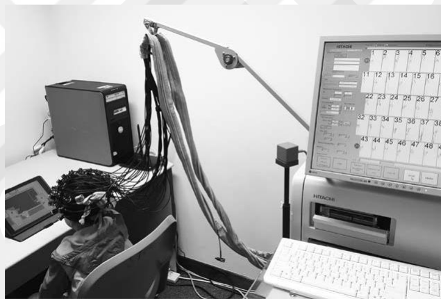
Figure 1.2 : An example of multi-channel fNIR spectroscopy [23].
