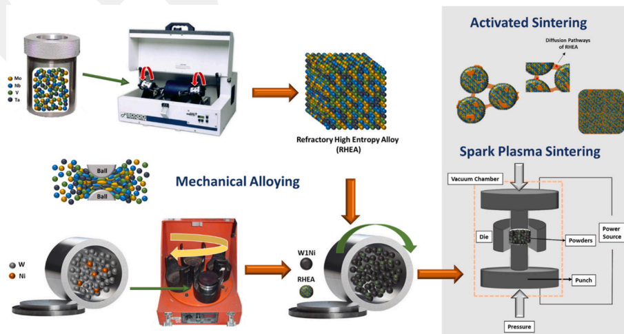
Fig. 1. Schematic representation for the production process of RHEA-reinforced W1Ni matrix composites.
