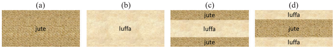
Figure 1: Designs of the test samples: green homogeneous (a) jute and (b) luffa fiber samples, and their hybrid (c) jute-luffa-jute (JLJ) and (d) luffa-jute-luffa (LJL) fiber samples.
